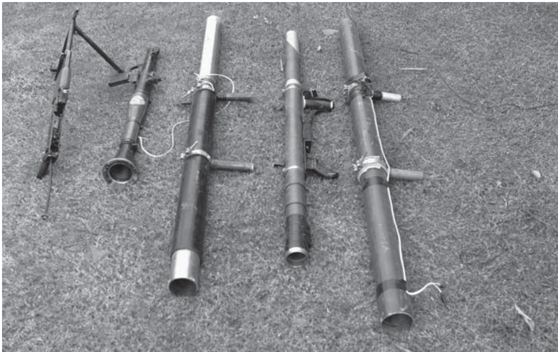
Three homemade Iraqi insurgent RPG-type rocket launchers captured by US Marines and Iraqi Special Forces in Fallujah in 2004. These launchers used light alloy or even PVC tubes and were good for only a few rounds before they became hazardous. To the left are a 7.62mm RPK (light machine gun version of the AKM assault rifle with its butt stock missing) and an RPG-7V antitank weapon. (US Marine Corps/SSgt Jonathan C. Knauth)
