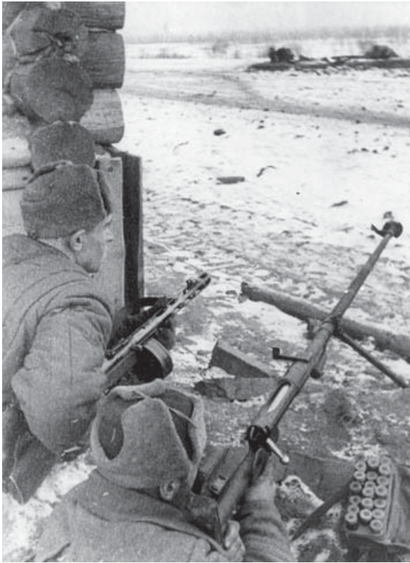
One of the most used Soviet antitank weapons during World War II was the massive 14.5mm PTRD-41 antitank rifle. It was heavy, cumbersome, and not very effective as a tank-killer. (Nik Cornish/STAVKA)
