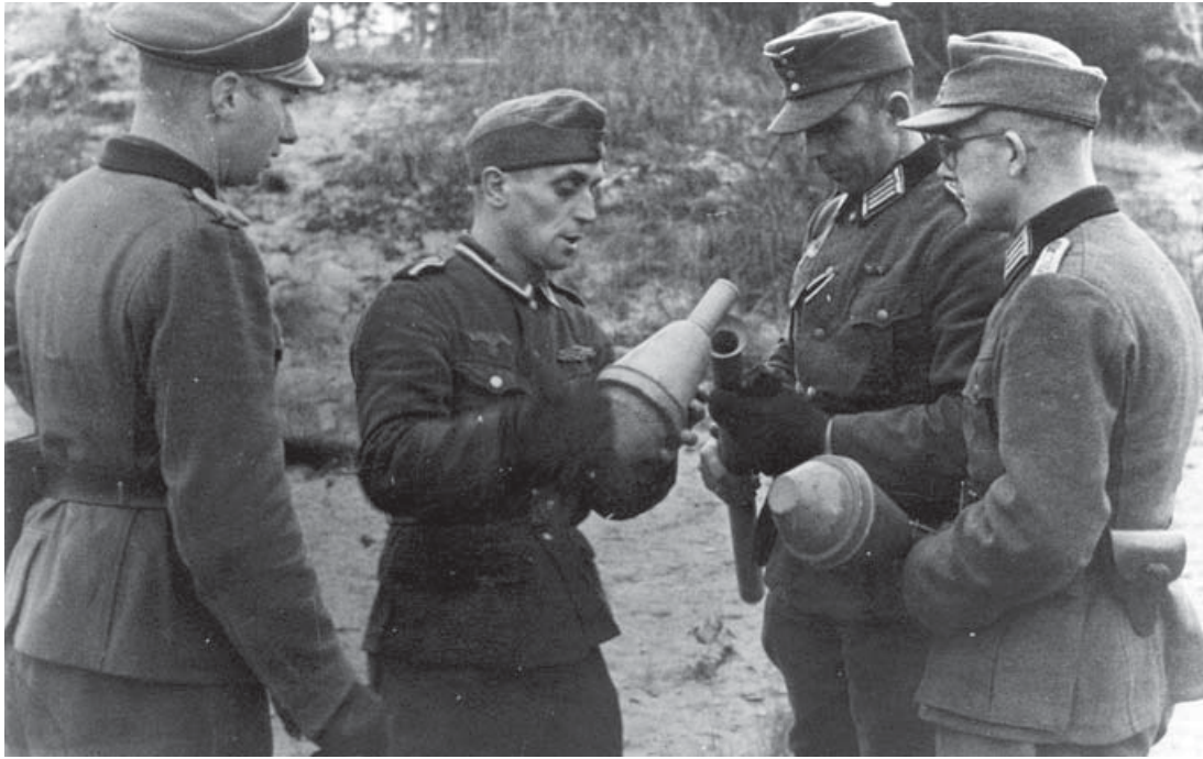
A German ordnance sergeant demonstrates the Panzerfaust 60 to officers. The Panzerfaust was not reloadable. The 140mm warhead could be removed, but the pre-loaded propellant charge was retained in the launcher tube. (Nik Cornish/STAVKA)
